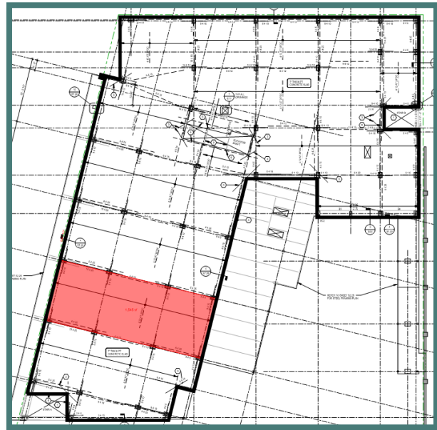
Figure 7: PT slab cost estimate takeoff (S2.2R – Second Floor Reinforcing Plan)
