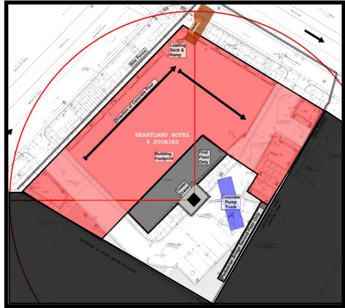
Figure 3.1: The site logistics plan for the PT slab construction process.
