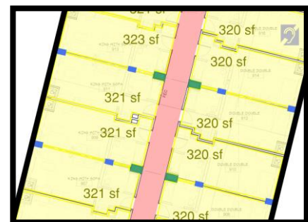
Figure 1.15: 9th story layout Green=mechanical shaft, Blue=columns
