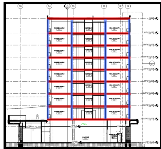
Figure 3.2: PT slab and columns in the Heartland Hotel.
